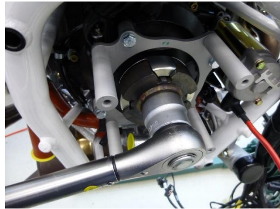
Fig. 4 - Tighten dog gear to 150Nm
