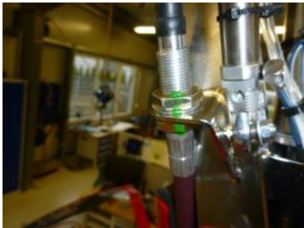
Fig. 2 - Push-pull control cable bulkhead attachment
