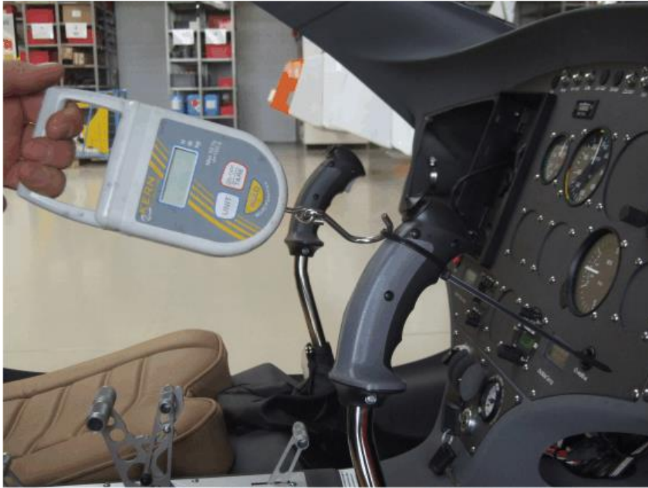
Fig. 1 - Measurement of rotor control friction
