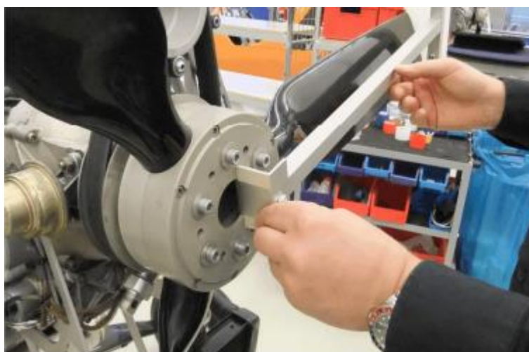
Fig. 2 - Propeller pitch adjustment and tool
