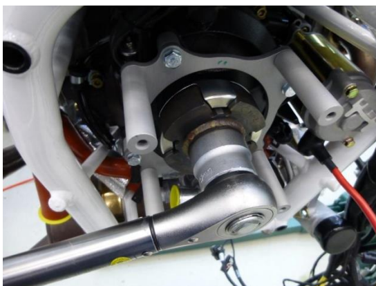
Fig. 5 - Torque dog gear with 150 Nm
