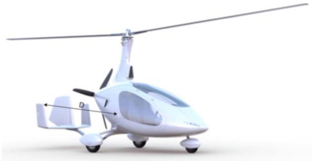
Fig. 1 - Measurement of Stabilizer Alignment (RH side shown)
