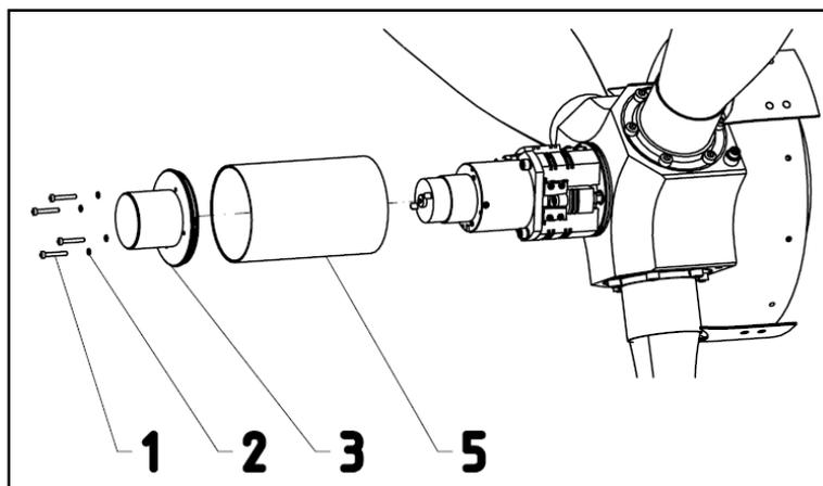
*Fig.5 Removal of covers of electro-mechanics*
