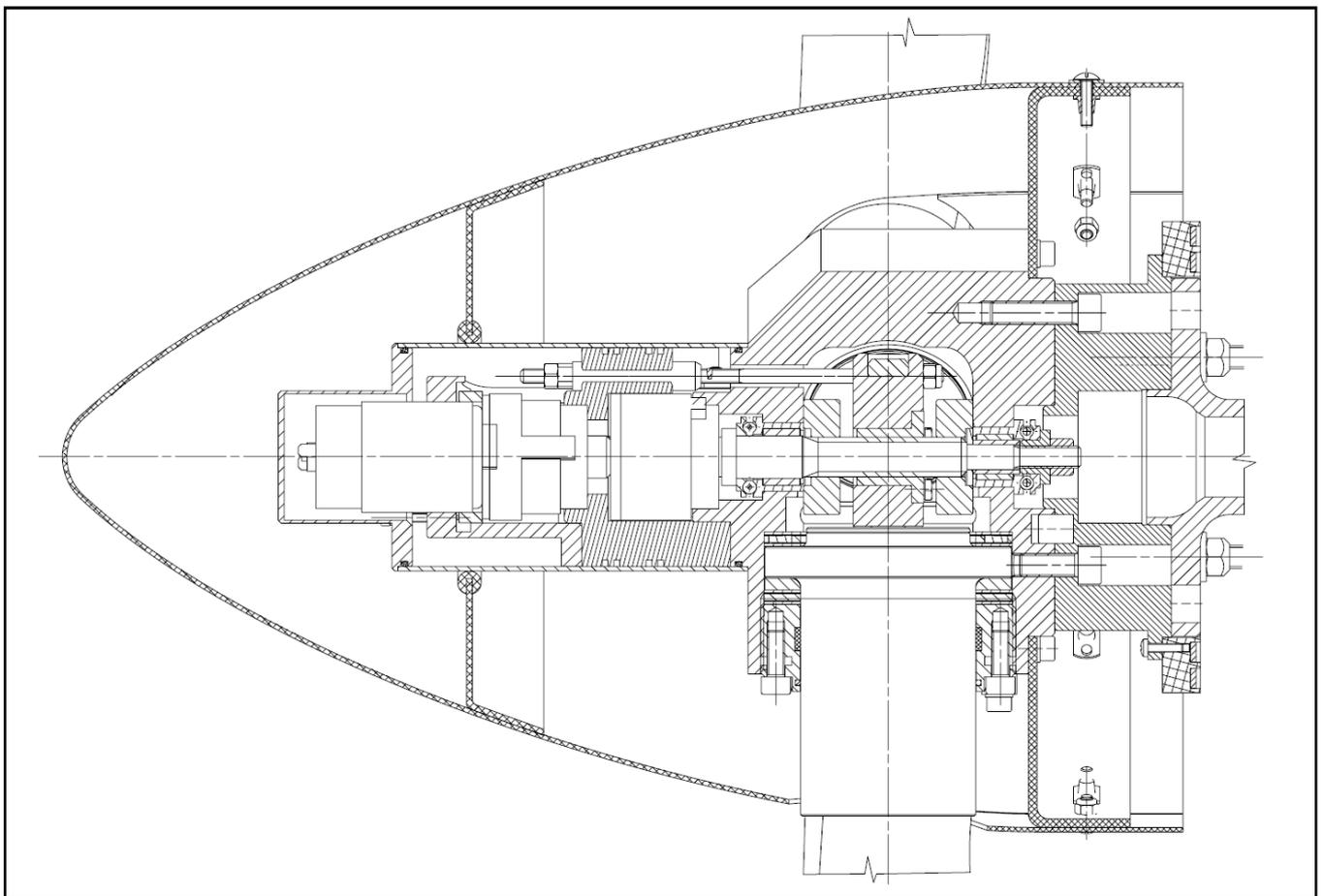
Propeller hub is made of aluminium alloy, and incorporates hydraulic mechanism for adjustment of blade pitch, and blade root pockets. Blades have mixed composition. Precisely machined wooden cores are covered in composite material, and their leading edges are protected by cast polyurethane or stainless steel inserts. Blade roots are set in aluminum alloy ferrules transferring the rotation and centrifugal forces into propeller hub.
