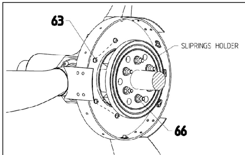
*Fig.2 Rear side of propeller installed on engine*
