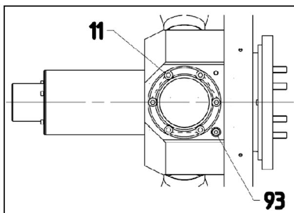
*Fig.3 Securing bolts on retention nuts and balance weights*
