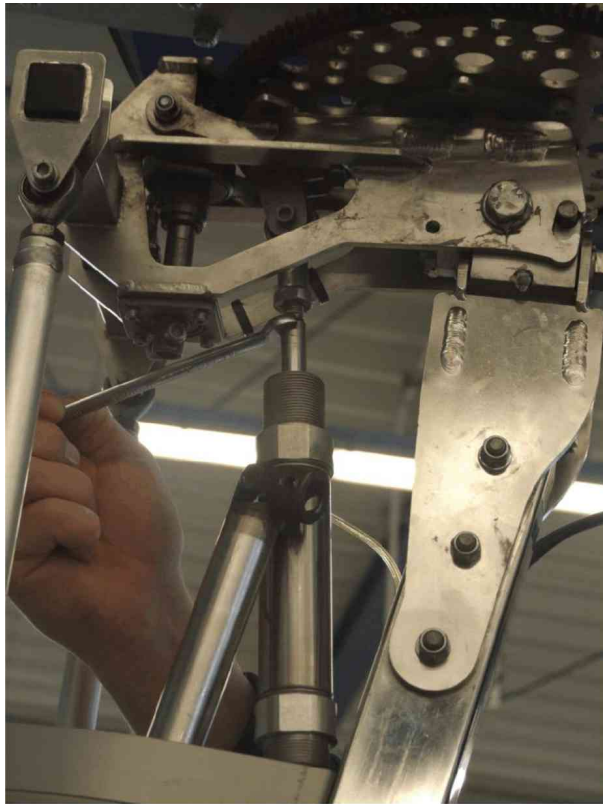
Fig. 1 - Disconnect rod end from ball joint (step 4)
