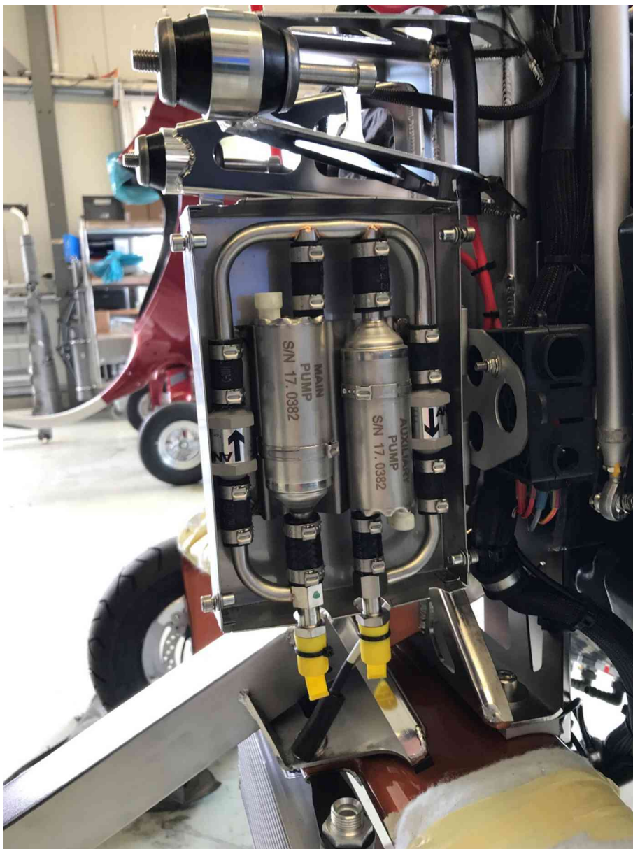
Location of pumps inside the Rotax pump box
