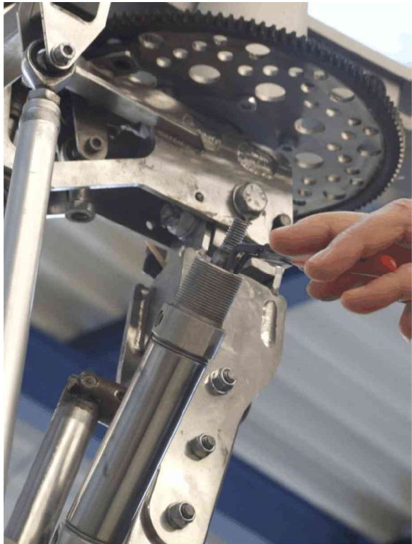
Fig. 2 - Remove circlip / snap ring (step 6)
