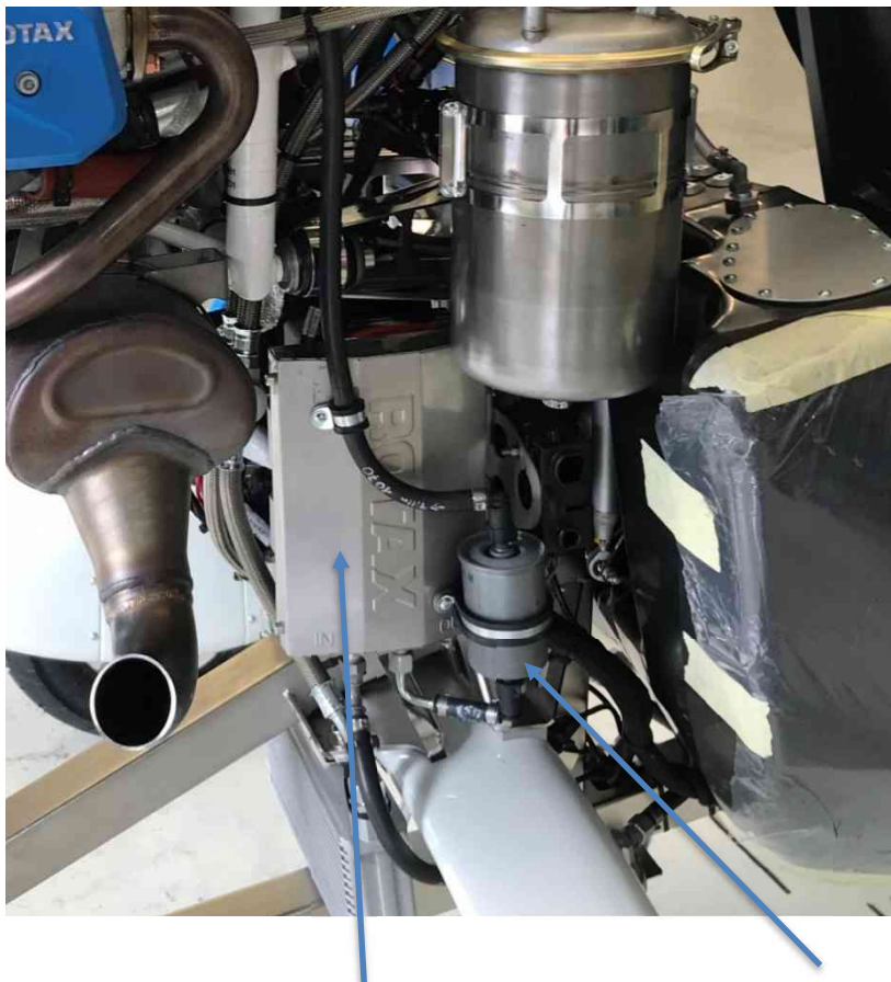
Location of fuel pumps (within this box) and quick-change fuel filter.
