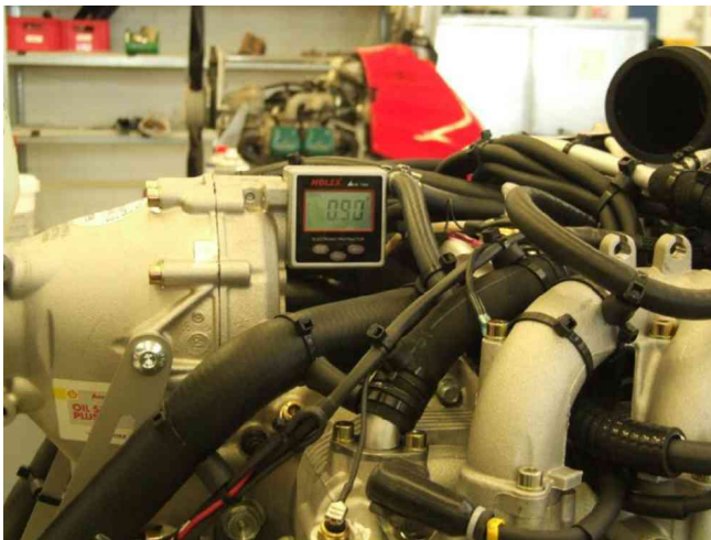
Fig. 4 - Measurement of thrust line angle
