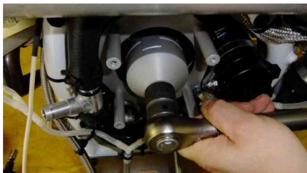
Fig. 5 - Torque dog gear with 140 Nm
