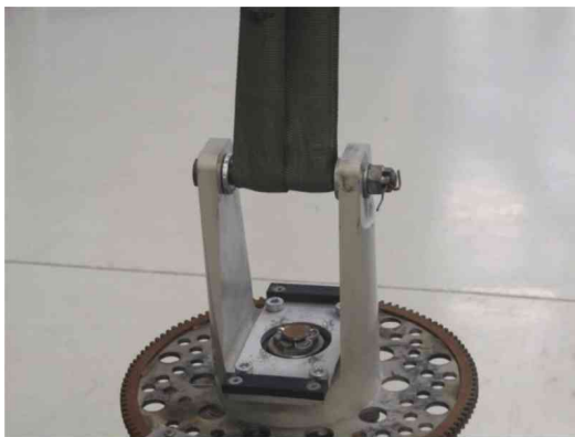
Fig. 1 - Lifting belt looped around teeter bolt
