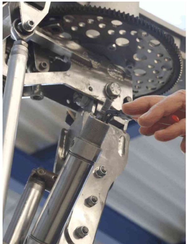
Fig. 4 - Re-connect ball joint and upper cardan hinge
