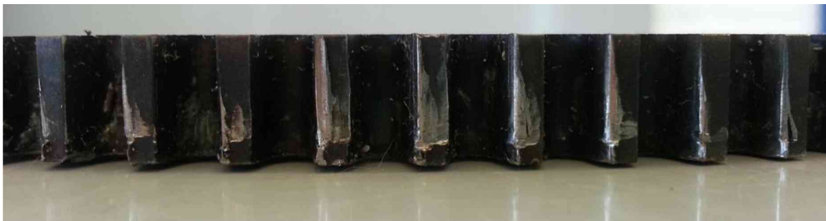
Fig. 1 - Wear Pattern (uneven)
