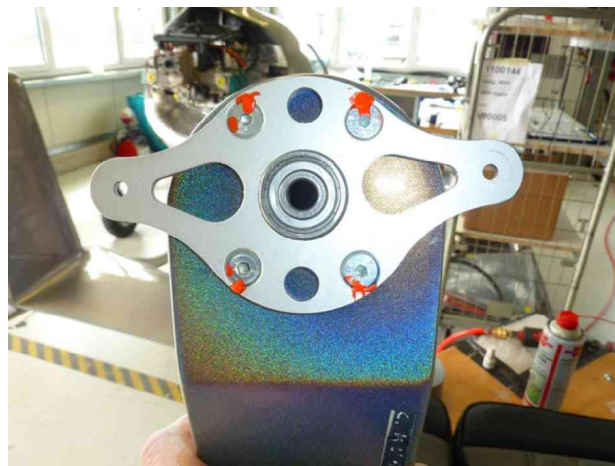
Fig. 3 - Flight control - Rudder control horn, note that the horn is offset so that the cables are equal length with the rudder offset 7.5deg to the right)
