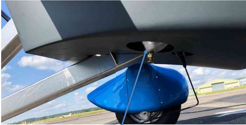
Location of gascolator drain point. Access is easy with body panels removed.
